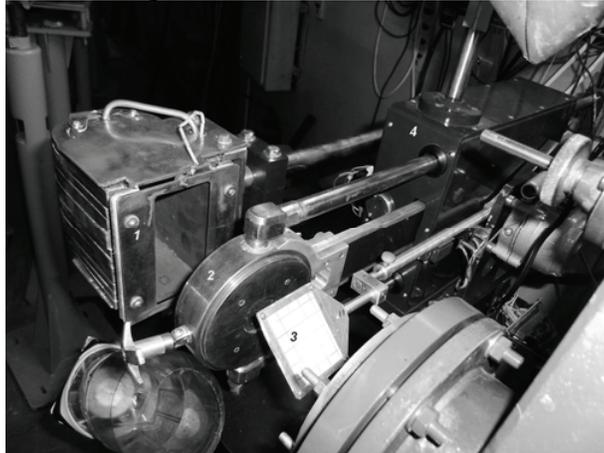
Fig.1 Experimental layout top view. 1 – Faraday cup, 2 – target device, 3 – luminofore frame for the beam spot size and position TV control, 4 – target remote control movement device.
