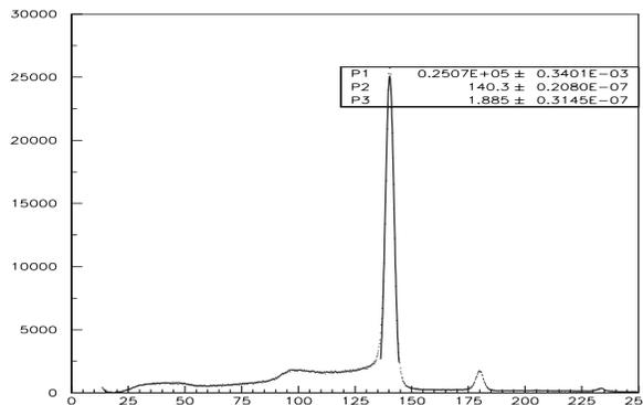
Figure 6. Energy spectra of irradiated material measured by Ge semiconductor detector.
