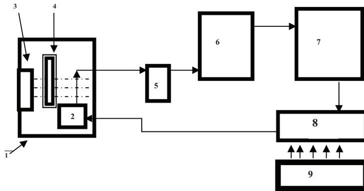
Figure 4. The water cooling system block-diagram. 1 – distilled water tank, 2 – water pump, 3 – water level sensor, 4 – electronic thermometer sensor, 5 – water pressure sensor, 6 – Faraday cup, 7 – target module, 8 – cooler radiator, 9 – electric fans.
