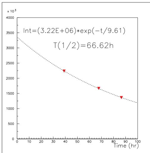
Figure 7. Dependence of radiation intensity from irradiated material on time.
