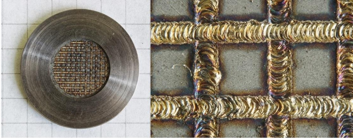
Fig.12. The target disk with a pressed molybdenum therein after the laser treatment (left), with x40 magnification (right).
