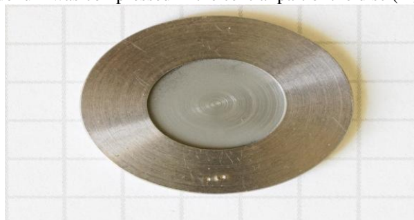
Fig.11. The disc target with the compressed natural molybdenum powder (the central circle).
