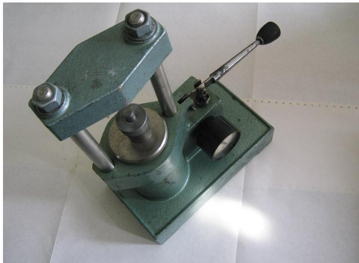
Fig. 5. A press with a matrix and a punch for pressing of molybdenum into a disk.
