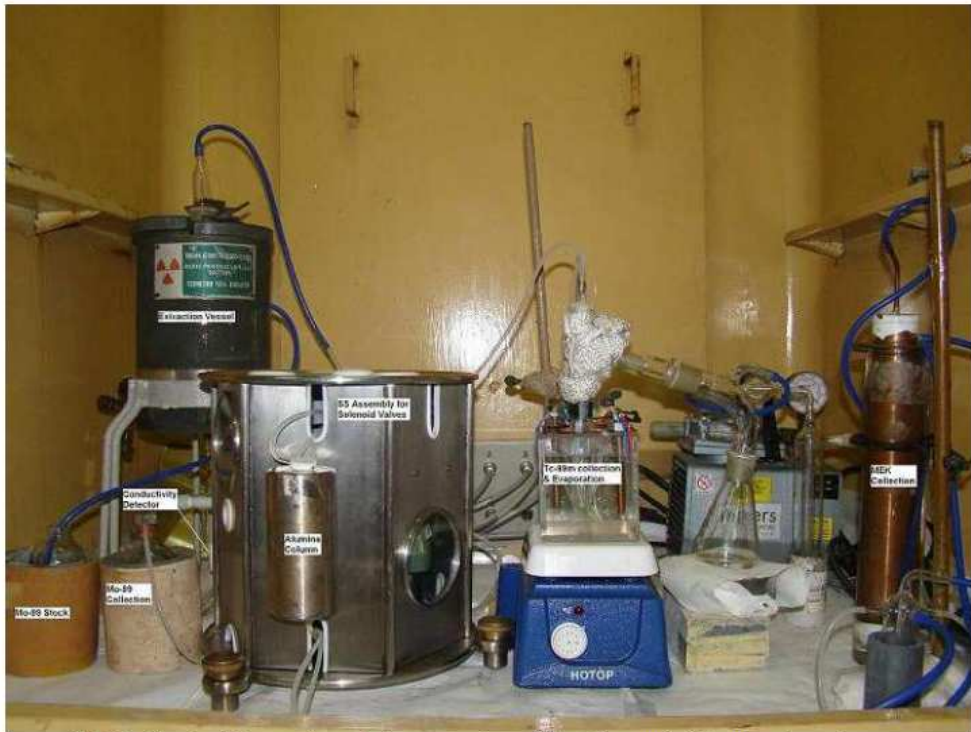
FIG. 1. Chemical Processing unit for separation of ^{99m}\text{Tc} from molybdenum using solvent extraction methodology.
