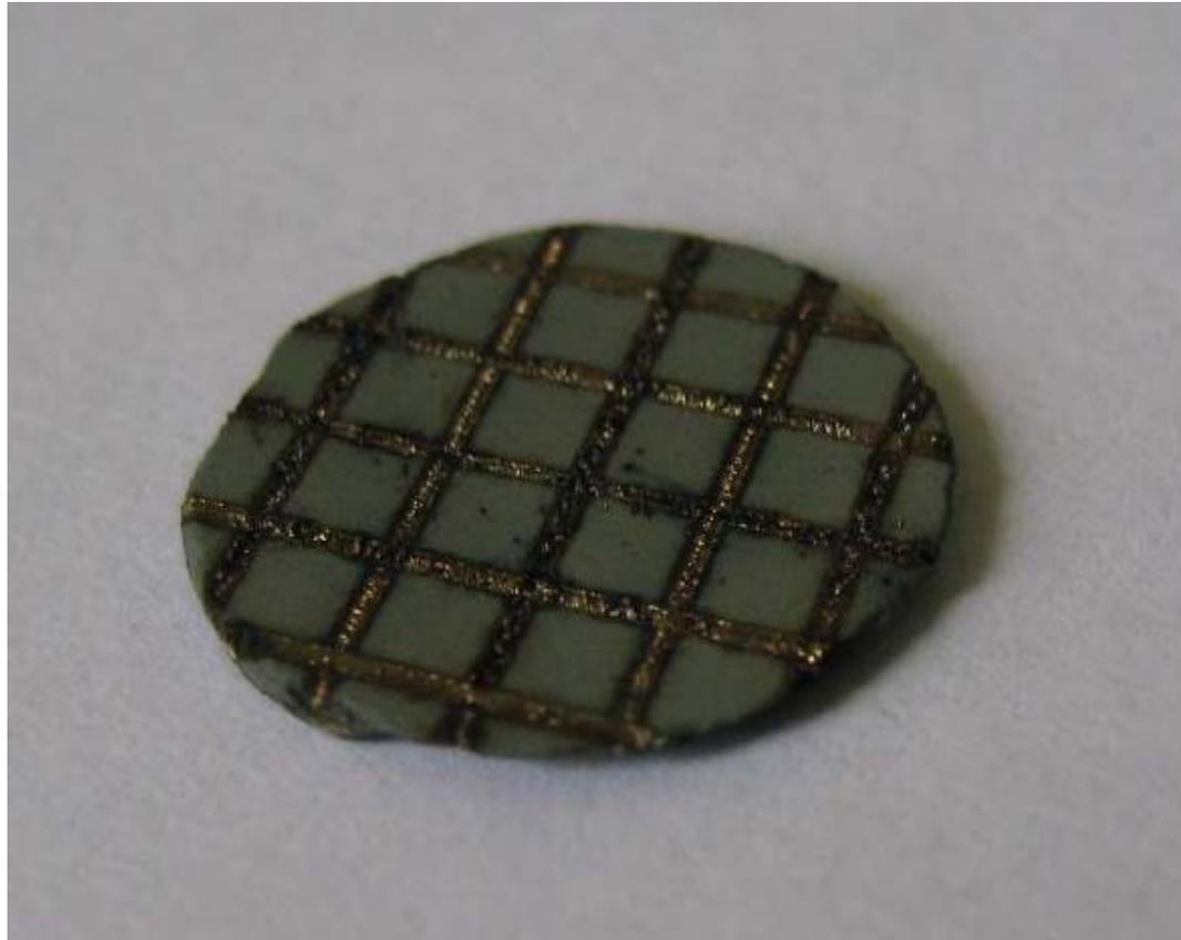
Then one side of that pellet was processing under **laser beam**. These grooves of the Mo powder became to **melted metallic solid state** are working **like metallic fixtures in concrete** providing enough **high mechanical strength** and **thermal conductivity**.
