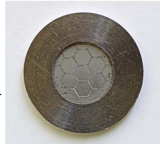
**Titanium disc with structured net and pressed Mo powder**
