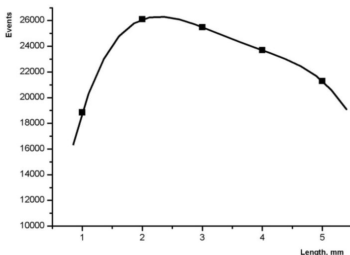
**Fig.4.** Dependence of the photon yield (in the energy range 9–20 MeV) from the converter thickness.
