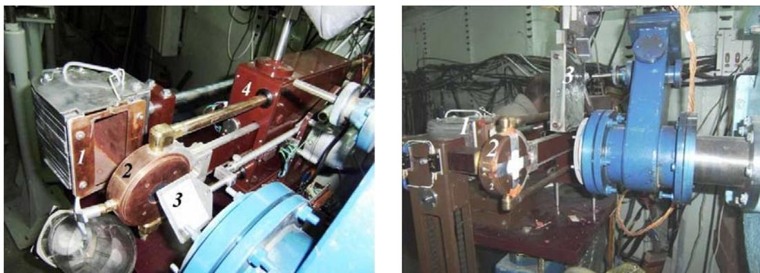
**Fig.2.** The experimental layout. 1 – Faraday cup, 2 – target moveable module, 3 – luminophore frame for the beam spot size and position TV control (on the left photo) or vibrating wire scanner module (on right photo), 4 – movement tool of target module.
