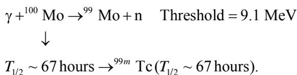
For this option the electron beam should be converted to a photon beam via bremsstrahlung. This method does not provide high specific activity and therefore does not allow building Mo/Tc generators but could cover the demand of regional and city clinics.
