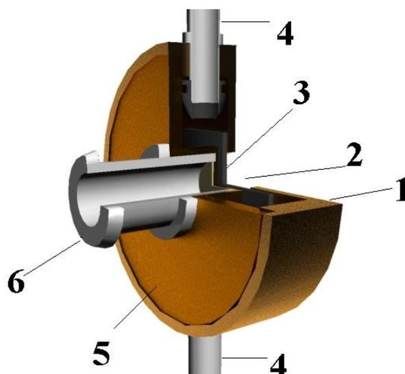
**Fig.3.** The target module. 1 – framework, 2 – beam entrance window, 3 – tantalum plate, 4 – water cooling pipes, 5 – cup, 6 – target capsule.
