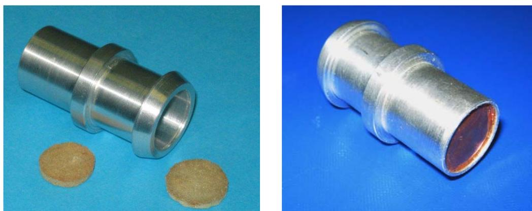
**Fig.5.** Target capsule for different tasks with pellets (left) and full amount (18 g) of pressed powder of  $\text{MoO}_3$  (right).
