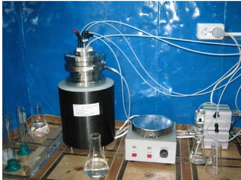
**Fig.10.** Main part of the centrifuge extractor complex.
