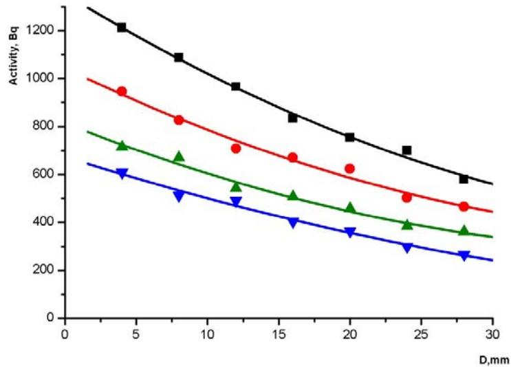
Fig.8. Measured obtained activity dependence on depth of natural MoO<sub>3</sub> target: ■ – 15.7 hours, ● – 37.8 hours, ▲ – 62.7 hours, ▼ – 84.3 hours after EOB.
