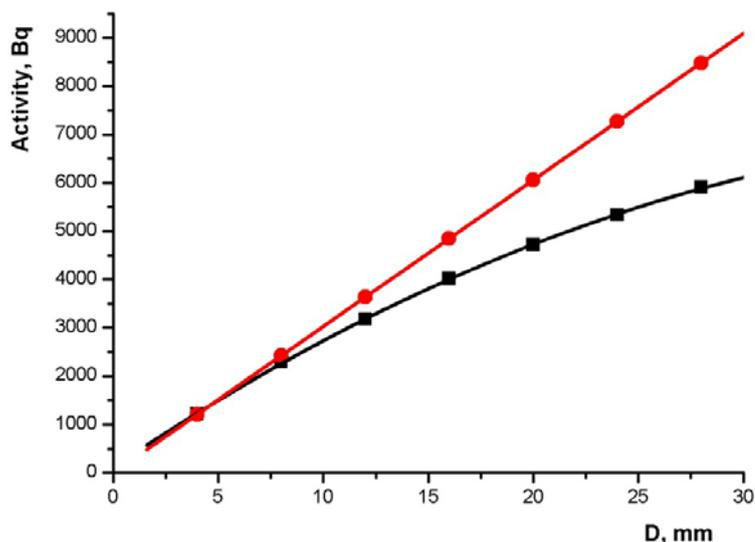
**Fig.9.** Measured integral activity (squares) and calculated integral activity assuming that the obtained activities of all pellets are the same (circles).
