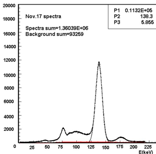
**Fig.6.** Energy spectrum from irradiated molybdenum.
