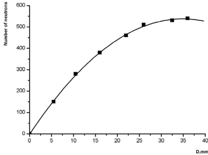
Fig.7. Calculated activity dependence on depth of natural MoO<sub>3</sub> target.
