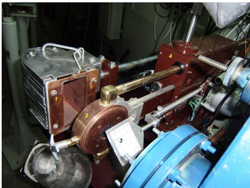
Fig.2. Experimental layout for irradiation under electron beam (top view). 1 – Faraday cup, 2 – target module, 3 – luminophore frame for the TV monitor beam profile, 4 – remote moving target module.
