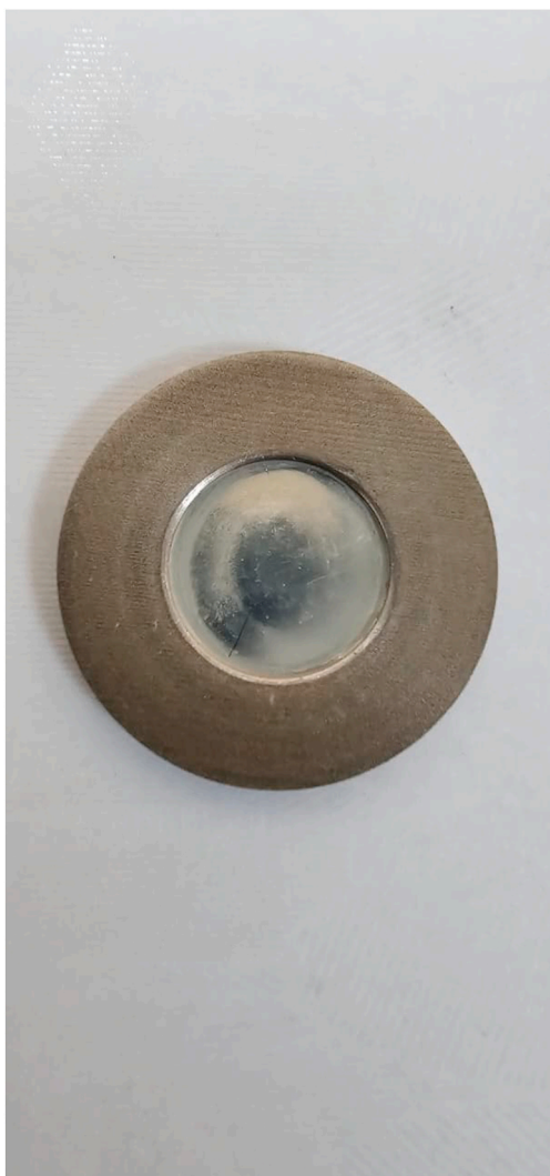
Fig. 3. Pressed natural zinc powder onto a niobium target holder.
