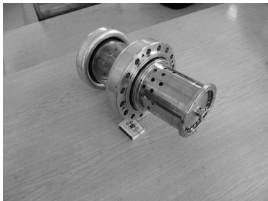
Fig. 1. Gun of linac LUE50 with the new metallic cathode.
