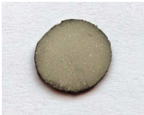
Fig. 13. Mo pillet with 10% of silberpowder compaund, pressed under 1000 kg force.
