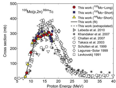
**Figure 8.** The cross-sections of  ${}^{100}\text{Mo}(p,2n){}^{99\text{m}}\text{Tc}$  reactions.
