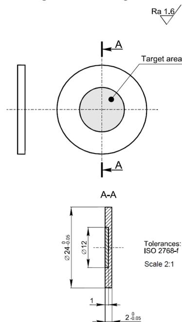
**Figure 9.** Solid target disc.
