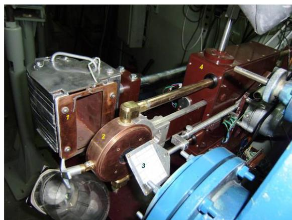
**Figure 3.** Experimental setup: 1 - Faraday cup, 2 - moveable target module, 3 luminore for the beam spot size and position along with video TV control and 4 target module moving system.
