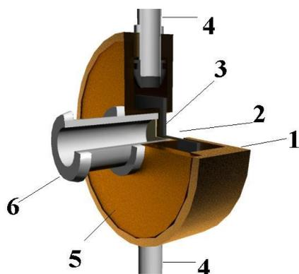
**Figure 4.** The body of the target module with identified components: 1 is the framework, 2 is the beam entrance window, 3 indicates the tantalum plate, 4 is the water cooling pipe, 5 is cup, and 6 is the target capsule (shown in greater detail in Figure 5).
