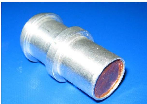
**Figure 5.** Target capsule with full amount (18 g) pressed powder of MoO<sub>3</sub>.
