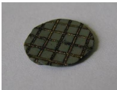
**Figure 10.** The target pellet processed by laser beam.
