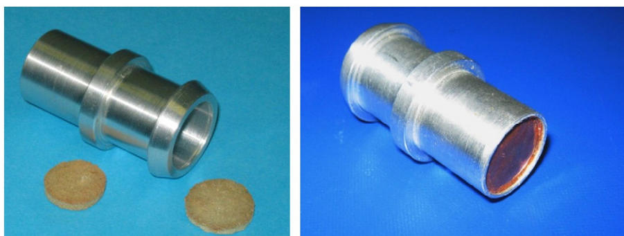
Fig. 6. The two modes of target preparation. The photograph on the left shows pressed pellets used in an aluminum tube whereas the photograph on the right reflects the same tube filled with the oxide powder with a copper film.
